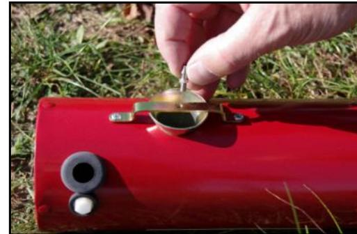
The propane nozzle will be screwed into the nozzle-bracket from the sound tube.
