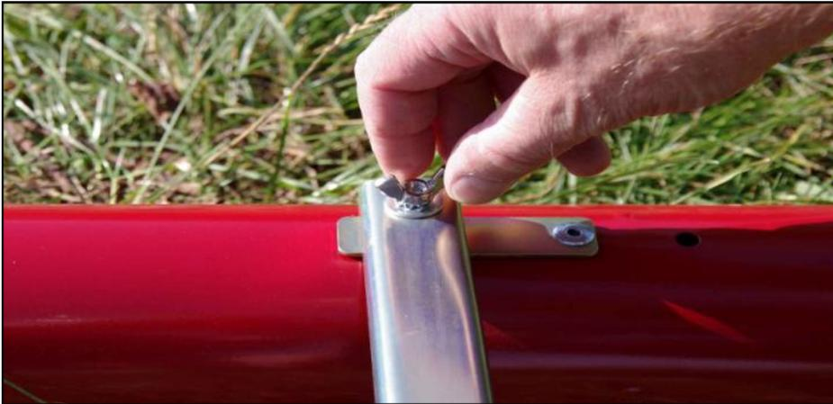
Once this is done the cross bar will be attached to the sound tube and tightened with the wing nut. Make sure that the cross bar is
