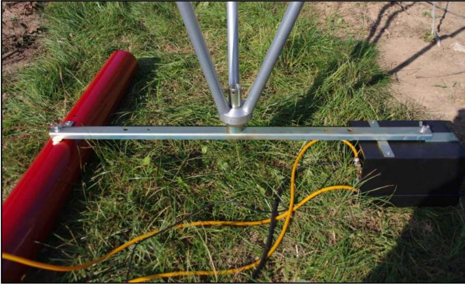
After all poles are mounted on the bearing block, the Purivox Carousel Triplex V can be turned over and put on the foot plates.
