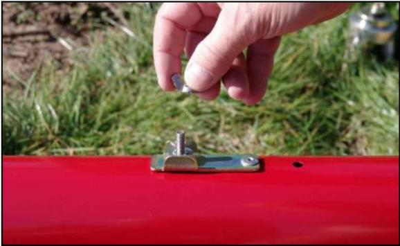
Remove the wing nut, toothed washer and the washer from the thread on the sound tube (106040).
