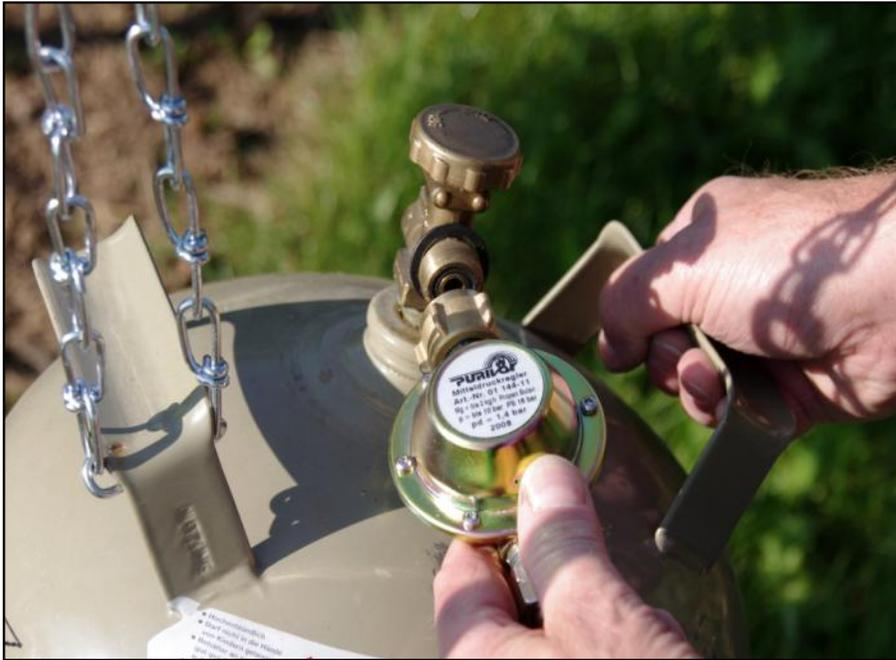
Screw the POL gas regulator (101660) on the propane gas bottle and connect the gas hose from the regulator with the gas hose (Gh-2) of the electronic unit. Take care that the two hoses are moved together completely.
