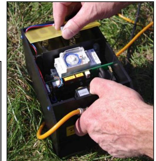
Open the lid of the electronic unit (108511) and make sure that the paper strip between the batteries and the contact board is removed.
